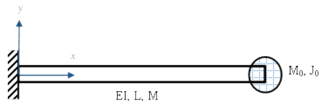
Figure 1 Schematic of a cantilever beam with an additional mass at free end
